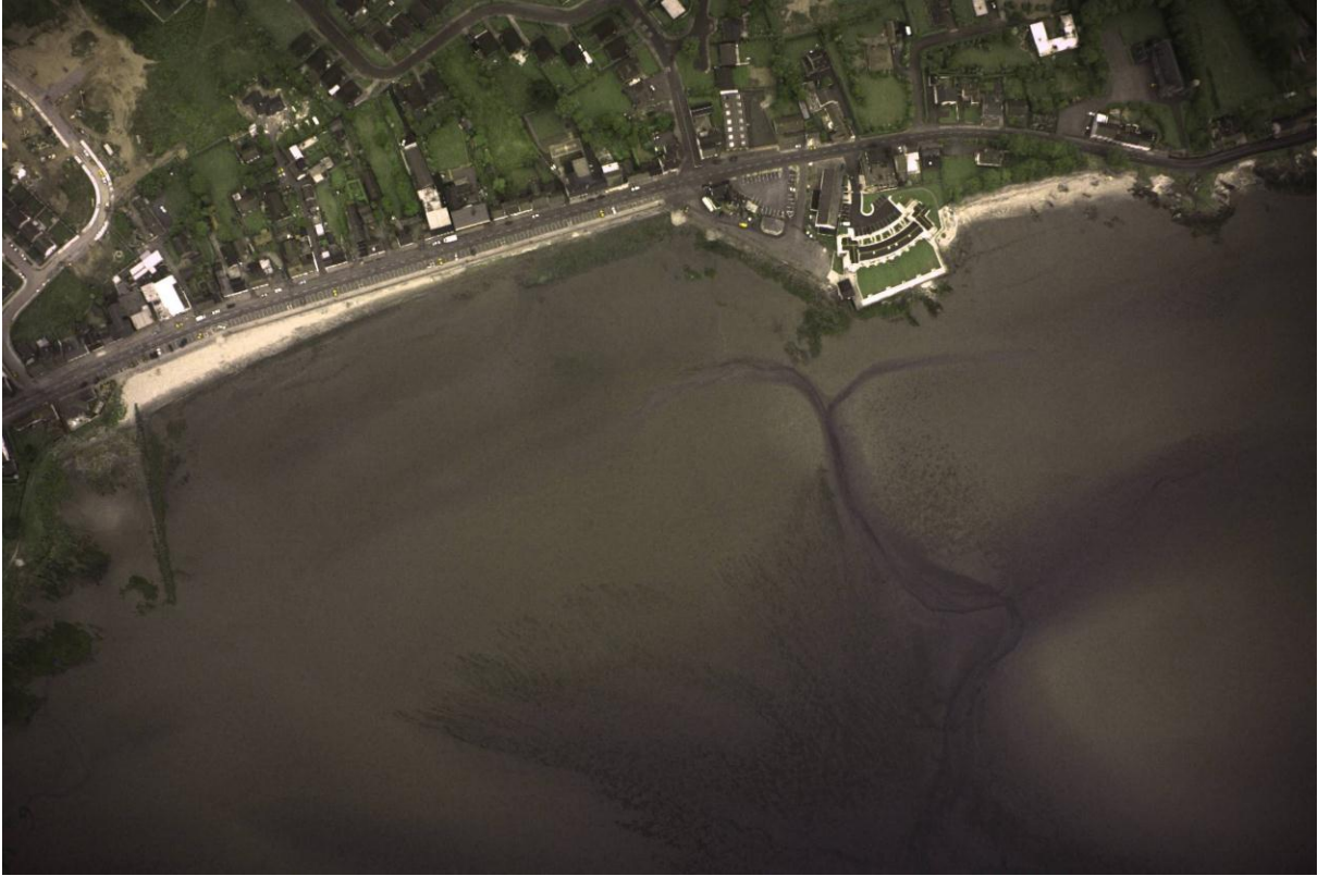
Photo 5: Beach 1998. Note eroded profile of beach at northern end, new car park, build up of material to the south of storm water outfall, and unchanged profile of Priest's beach.
