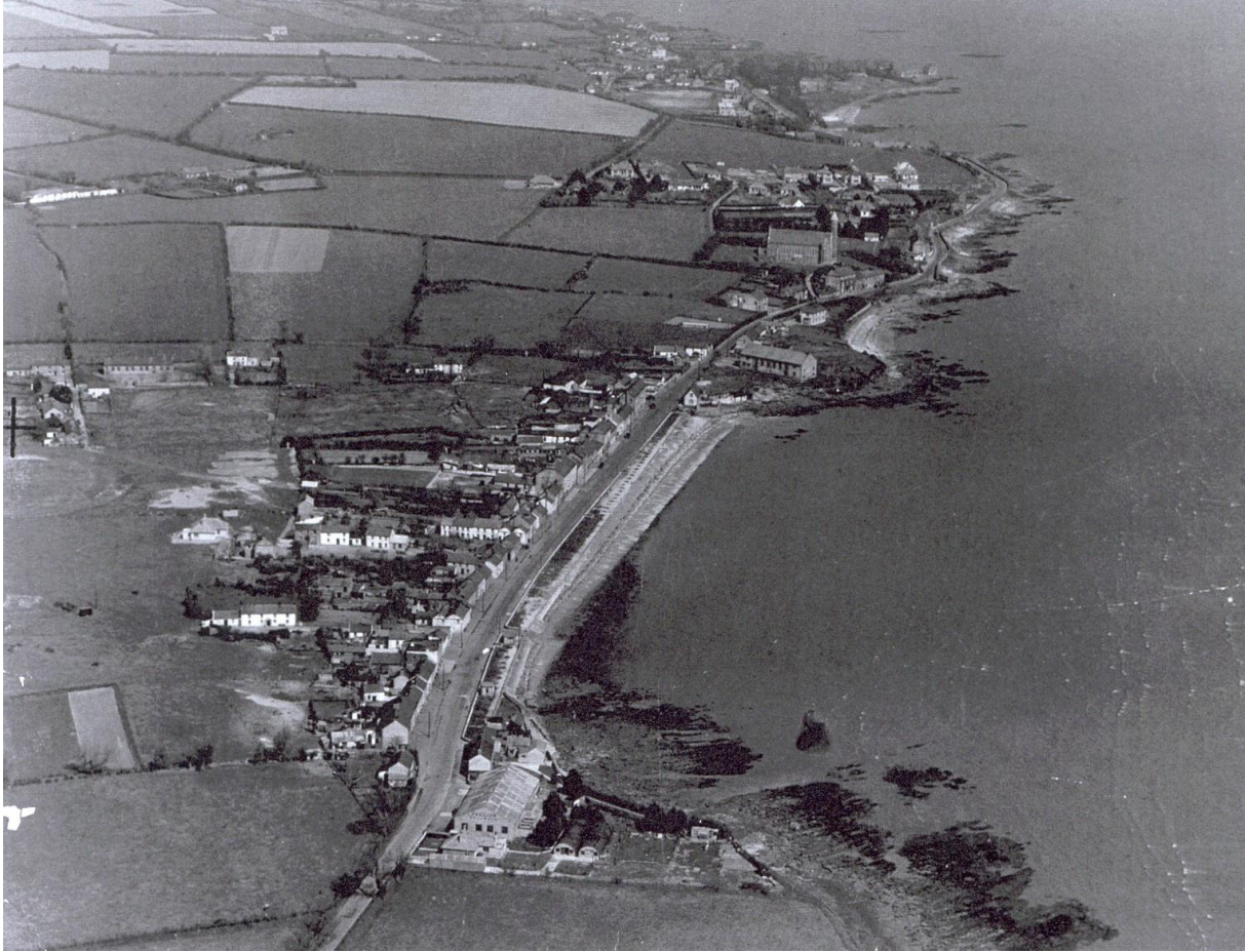
Photo 2: Beach circa 1950. Note beach width wider at north than at south indicating possible accretion at this location. Also note High Water mark as indicated by feint black line running along the beach, narrowest at south and getting progressively wider to the north.
